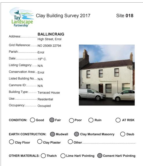
**ASSESSMENT:** The owner confirmed mudwall which is visible at the rear of the property. It has a modern cement render and window alterations.
