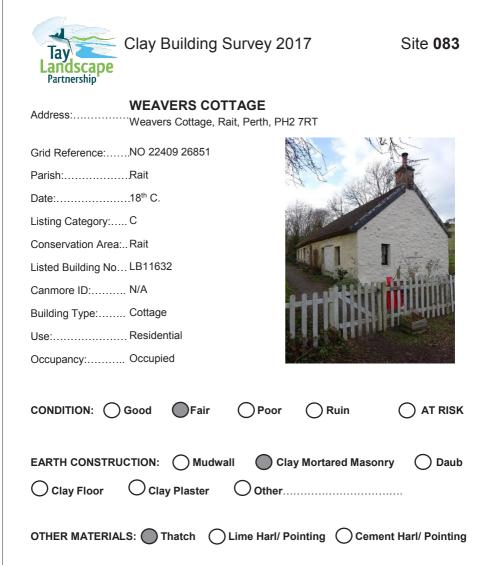
**ASSESSMENT** 18<sup>th</sup> century pair of cottages, united into one. The cottages have a continuous thatched roof, thatched in reed. Single storey whitewashed rubble. Wallhead slopes with ground. Brick chimneys. Highly likely to be clay mortared masonry, given age, location and precedent
